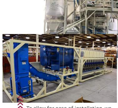
To allow for ease of installation, we mounted these on 3 skid based systems and prewired each skid to minimize the amount of on-site work.
